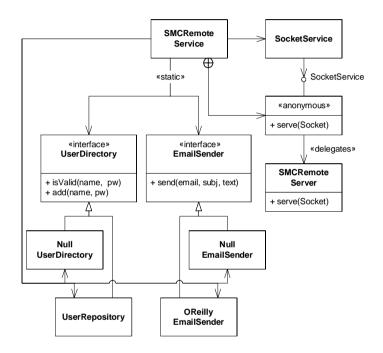
Figure 12-12 High level structure of SMCRemoteService
