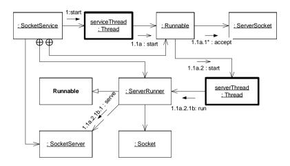
Figure 12-11 SocketService Object Diagram
