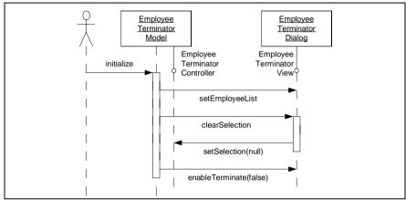
Figure 6-7 Interaction between the Model and Dialog
