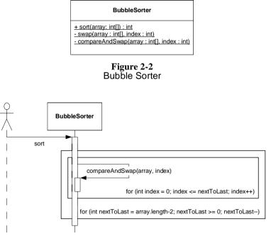
Figure 2-3 Bubble Sort Sequence Diagram
