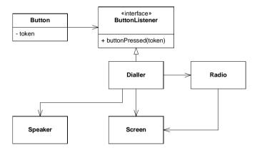
Figure 2-8 Isolating Button from Dialler
