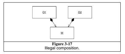
• The owner is reponsible for the lifetime of the ward. If the owner is destroyed, the ward must be destroyed with it. If the owner is copied, the ward must be copied with it.
