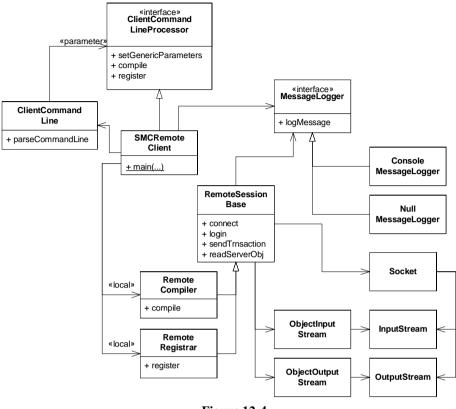
Figure 12-4 SMCRemoteClient Static Structure
