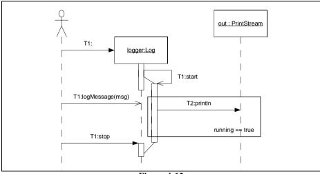
Figure 4-12 Multiple Threads of Control
