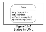
slightly different meaning. Any transition that exits a state will invoke the exit action (if any). Likewise any transition that enters a state will inoke the entry action (if any). Thus, in UML, a reflexive transition like Figure 10-3 invokes not only myAction, but also the exit and entry actions.
