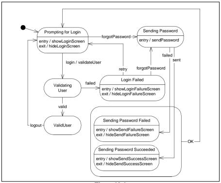
Figure 10-1 Simple Login State Machine
