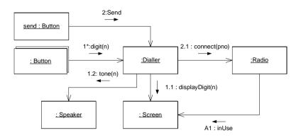
Figure 2-6 Cell Phone Collaboration Diagram
