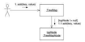
Figure 1-5 Collaboration Diagram of one case of TreeMap.add
