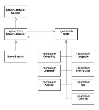
Figure 12-16 Three Level Finite State Machine.
