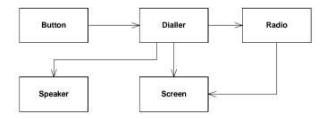
Figure 2-7 Cell Phone Class Diagram
