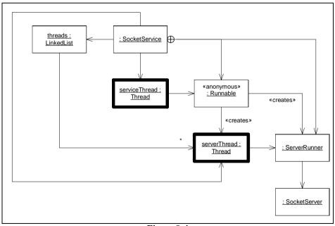
Figure 9-4 SocketService Object Diagram
