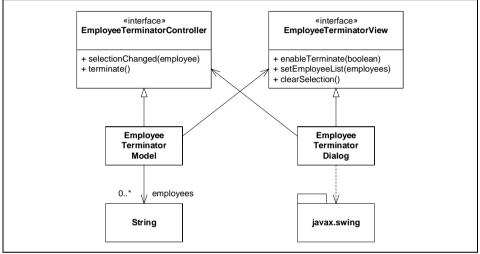
Figure 6-6 Isolating GUI from Data Manipulation
