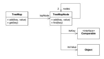
Figure 1-2 Class Diagram of TreeMap
