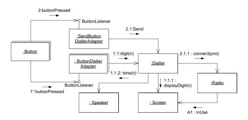
Figure 2-10 Adding Adapters to the Dynamic Model
