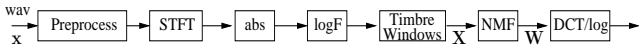
Fig. 1. Calculation of the features used for the statistical model of musical genres
